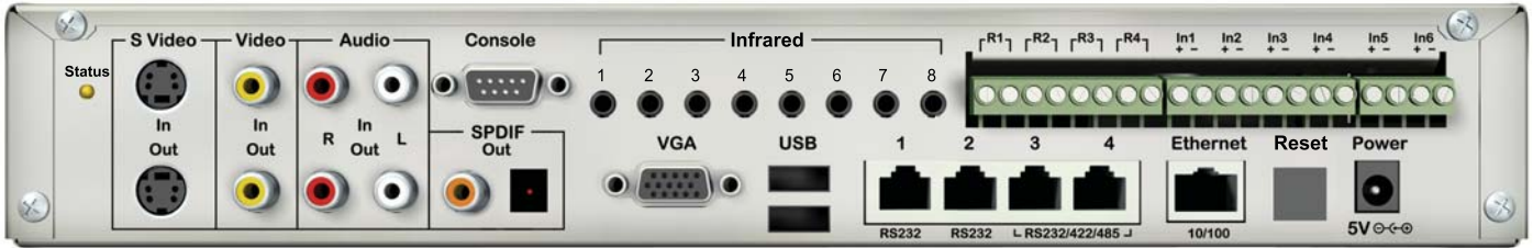
ControlBox CB-101-S, CB-102HD-S Back Panel
